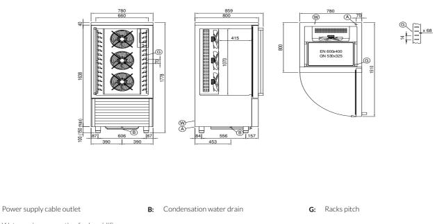
W: Water mains connection for humidifier - 3/4" female. Unloading not required
