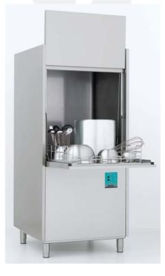
Thanks to the  $70 \times 70 \text{ cm}$  rack and the 85 cm open door clearance, the Domina LOD 402 meets all your requirements. Detergent and rinse aid dispenser are optional, both can be set and adjusted electronically from the control panel. Four wash cycles of 2, 4, 6 or 8 minutes.
